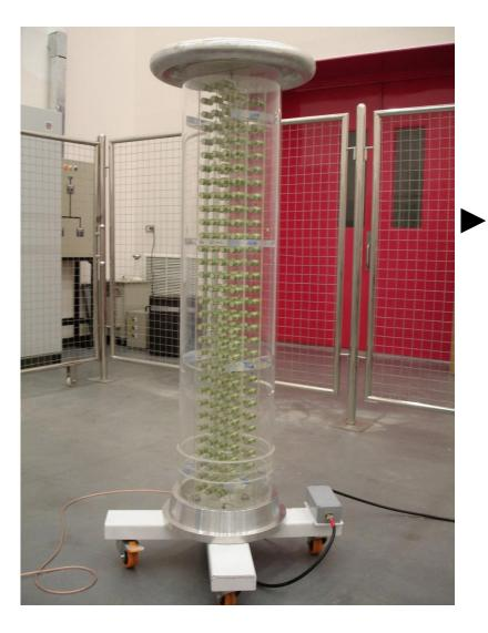
250 of 0.1 pF are serial-connected (Total = 400 pF)
