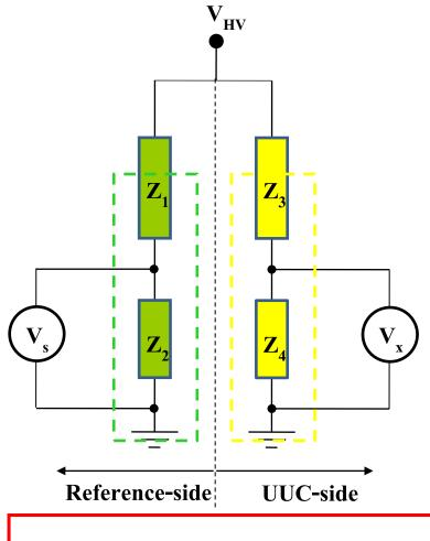
High voltage is applied to both, the reference measuring system and the unit under calibration (UUC), while the output of both measuring system are simultaneously measured and compared to scale factor of the UUC.
