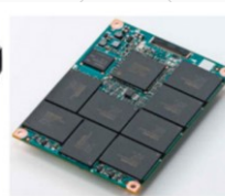
Memory based hard drive (SSD)
