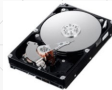
Traditional Hard disk mechanical drive
